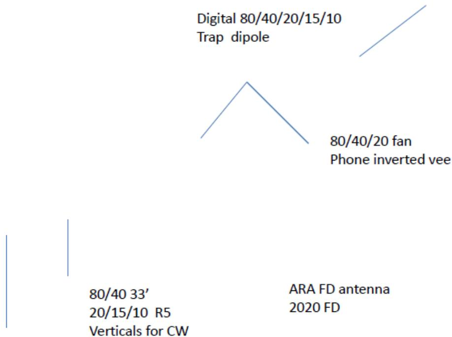
The antenna clusters need to be in a line to achieve polarity isolation across all bands and combinations of antennas. Then use verticals for the first cluster, inverted vees (helps with bandwidth on 80 meters and tuning end points for isolation) for a second cluster, and a trap dipole for the 3<sup>rd</sup> position.
