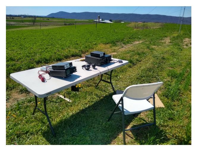
This is the setup for receiving on a Yaesu FT-950 near the inverted vee (the FT-991A is also setting on this table in this photo). A small 12V battery under the table was used to power the FT-950 for most tests to ensure no signal coupling over power cables. The bandpass filters used to eliminate out of band noise and signals are visible behind the FT-991A, and the small portable oscilloscope is visible near the FT-950.
