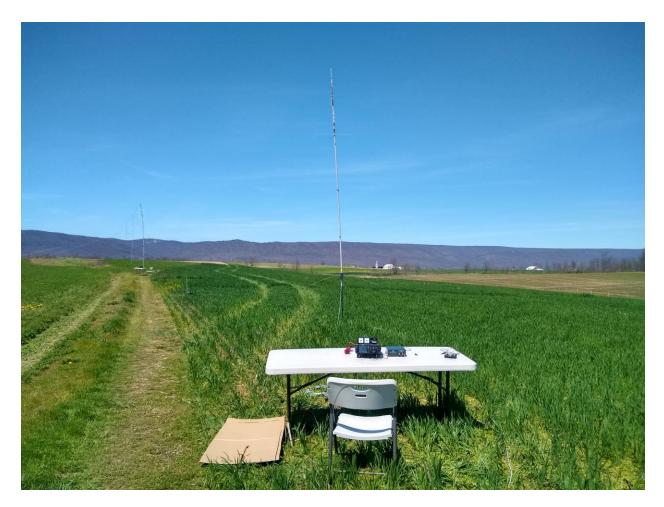
This was the setup for transmitting CW at 100 watts on the nearby verticals using a Yaesu FT-991A. A small generator is faintly visible about 100 feet down the lane. A contest keyer sent a test signal and station ID repeatedly during each test sequence.
