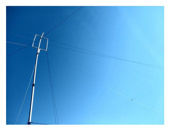
The independent end points of the legs of the inverted vee for each band allowed each band to be independently optimized for isolation and was necessary as shown in the picture. Once this isolation was achieved, CW interference from the verticals into the phone inverted vees resulted in imperceptible interference with 50 to 100 KHz separation on 80 or 40 or 20 meters.
