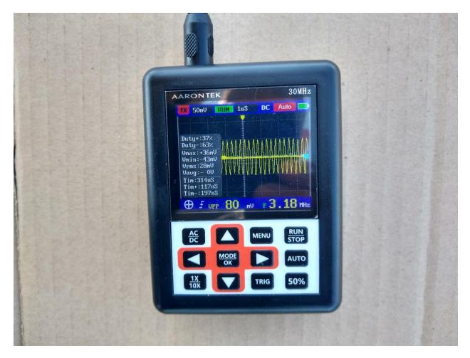
This is a small portable battery-run scope used to measure interference signal levels and used to guide tuning the antenna positioning to maximize isolation.
