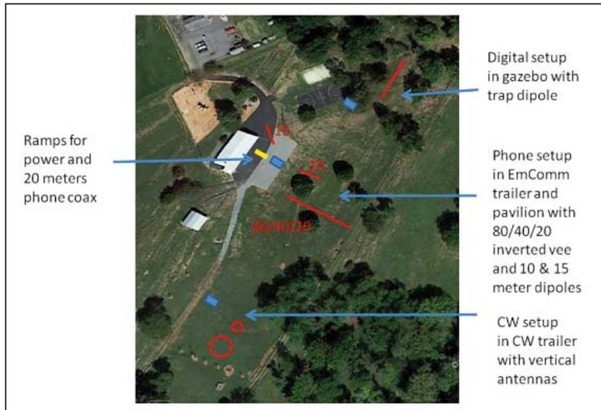
**Figure 1 — W3CWC Field Day 2021 antenna layout.**
