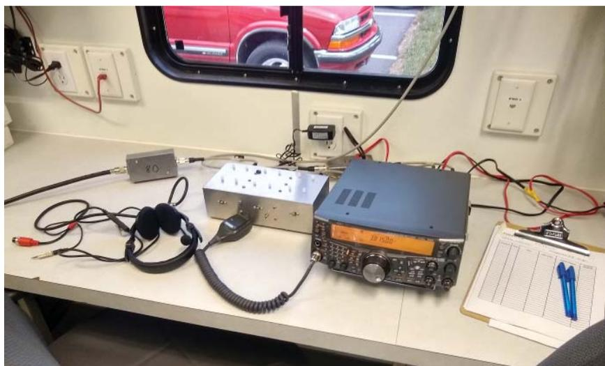
**Figure 3 — The 80-meter phone setup for the TS-2000. The larger aluminum box is the USRX filter for 80 meters and the smaller aluminum box is a band-pass filter for 80 meters.**
