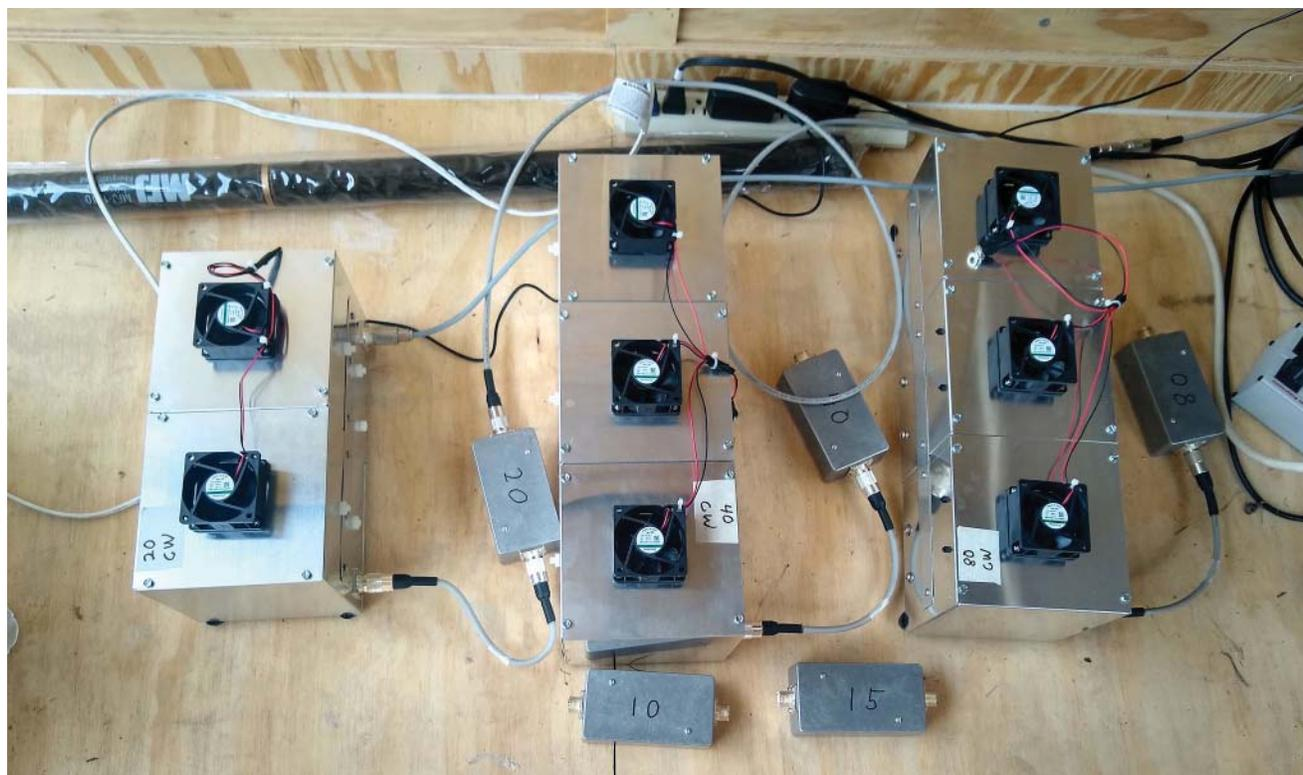
**Figure 5 — The CW filter bank.**
