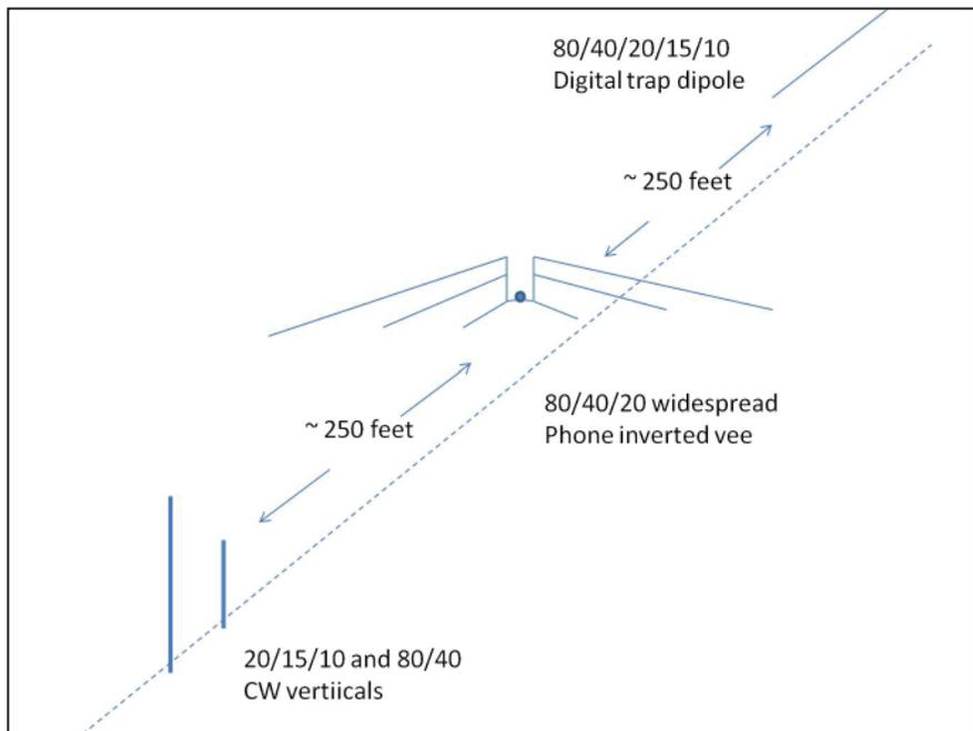
**Figure 2 — W3CWC Field Day 2021 antenna diagram.**
