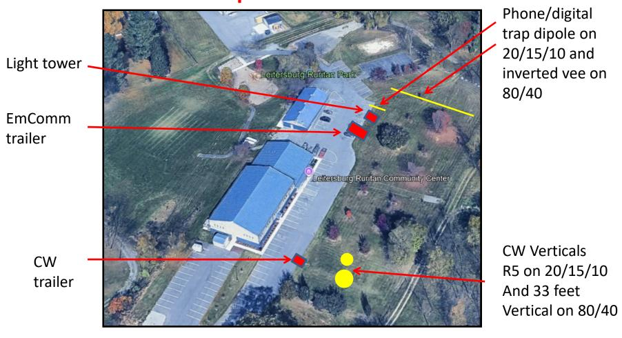
The phone/digital dipole and inverted vee are placed to be perpendicular To a line drawn to the CW verticals to achieve cross-pol isolation
