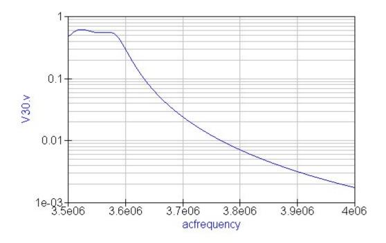
This is the response of the 3-stage pre-selector for the 80 meters CW band from QUCS simulation/analysis. There is 4 to 5 dB of insertion loss in the CW band. The loss in the phone band reaches 30 dB at about 3.680 MHz and ramps to almost 60 dB at 4 MHz.
