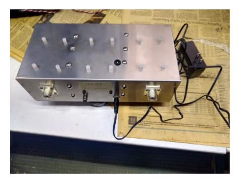
These are pictures of the completed 40 meters USRX filter. The toggle switch on the front of the chassis is used to bypass the filter. The 3 slots for the variable air capacitors are visible on the front. On the back of the chassis are input/output UHF connectors, a 12 VDC jack with the 12 VDC power plug, and a phono jack for the TX/RX control cable to the rig. An LED to indicate status is on the top of the chassis in a rubber grommet.
