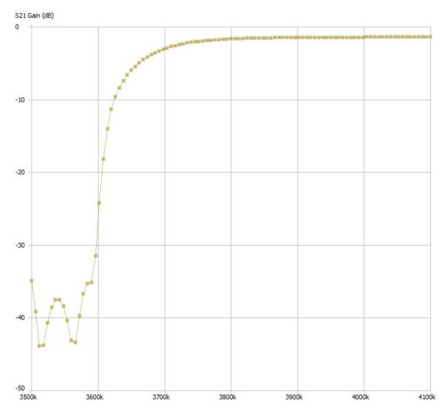
This is the measured response of the 80 meters USRX filter. The CW band is suppressed by about 35 to 45 dB, but the phone band only sees 1 to 2 dB of loss over most of the band. The 3 notch filter resonance points are visible between 3500 and 3600 KHz with one at about 3580 KHz that forms a shift in the curve, and the other 2 forming clear sharp notches around 3510 and 3560 KHz.
