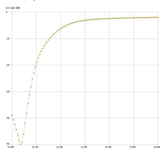
This is the measured response for the 20 meters filter for phone operation measured from 14.0 to 14.6 MHz.
