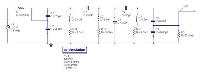
This is a schematic for a 3-stage high-Q preselector for the 80 meters CW band (R11, R12 and R13 are models for the resistance of the inductors). The internal impedance is about 5000 Ohms, and capacitive dividers at the input/output provide matching to 50 Ohms. C1, C5 and C6 can be composed of a fixed capacitor in parallel with a trimmer capacitor to support precise tuning.
