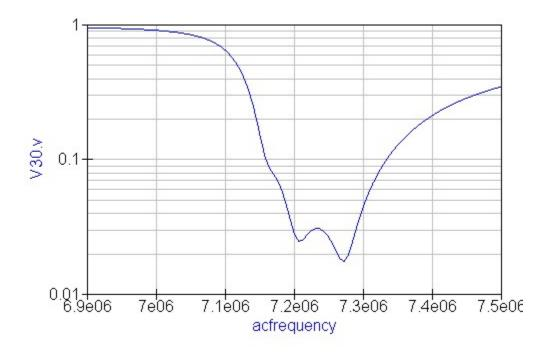
This is a 40 meters USRX filter response (simulation) from 6.9 to 7.5 MHz for CW operation with notches on the phone band and a band-pass bump on the CW band. The band-pass bump and ultra-sharp transition are clear on the lower side of the notches going from the phone band down in frequency to the CW band. This filter uses inductive coupling between 3-stages of notching.
