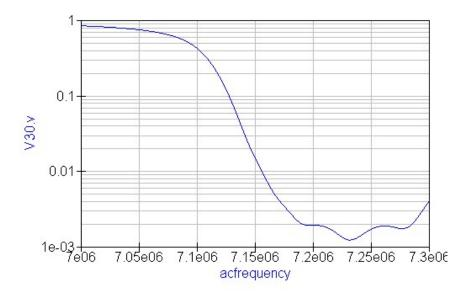
This is the simulation result for a CW filter with a 5-stage notch design which achieves around 50 dB of suppression over most of the phone band with only several dB of loss over most of the CW band.
