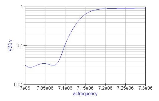
The simulation result with detailed modeling shown here is fairly close to the measured result shown early in the paper for the prototype filter. About 1 dB of loss should be added to account for the RF transformers which results in a good match from 7.2 to 7.3 MHz of about 2 dB of loss. And the loss in the CW band is about 27 to 31 dB with measured results of 25 to 30 dB.
