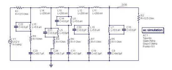
The schematic of the 5-stage notch filter shows 12.5 Ohms input/output impedances which would be matched to 50 Ohms with RF transformers. Small inductors of 200 nH couple the stages to provide a band-pass bump below the stop-band.
