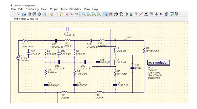
This is a model of the 40 meters USRX filter with resistors added to model inductor Q, and stray capacitance and stray inductance added to generate accurate results and to clarify mechanical design issues affecting performance.
