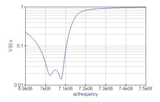
This is a 40 meters USRX filter response (simulation) from 6.9 to 7.4 MHz for phone operation with a notch on the CW band and a band-pass bump on the phone band. The band-pass bump and ultra-sharp transition are clear on the upper side of the notch going up in frequency from the CW band to the phone band. This filter uses capacitive coupling between 3-stages of notching.
